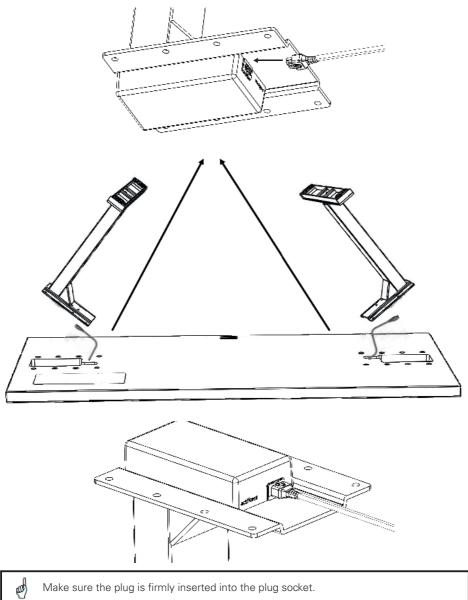
Do not pull the connectors further out of the tabletop.
