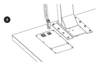
Keep in mind that the table which you are assembling is height adjustable. The cables of the electrical components must be able to freely follow the movement of the table.
